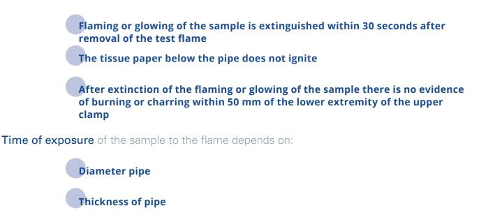
The greater the diameter or thickness, the greater the flame exposure time. **For this reason a ranging Masterbatch dosage is suggested.**
